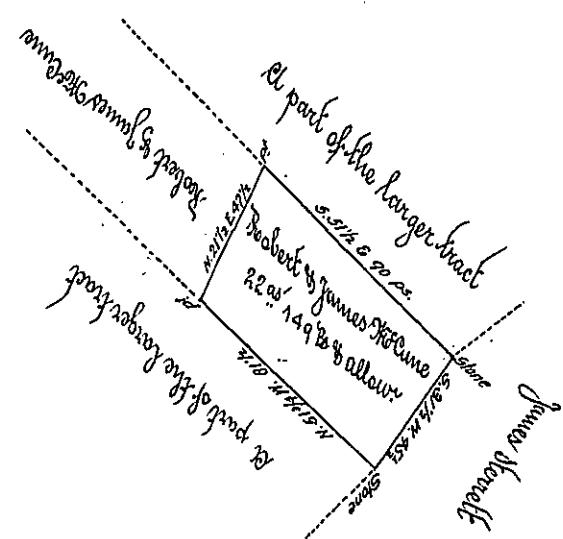
A Draught of a tract of Land Situate in Newton Township Cumberland County Containing 22<sup>ac</sup> 149<sup>ft</sup> <sup>6</sup>/<sub>8</sub> allowance of six per cent for Roads &c. It being part of a larger tract of 23<sup>ac</sup> 79<sup>ft</sup> <sup>6</sup>/<sub>8</sub> allr. Surveyed in pursuance of a warrant granted to Robert & James McCune dated the 20<sup>th</sup> Day of October 1766. Surveyed and Divided 22<sup>nd</sup> Day of March 1811 —
